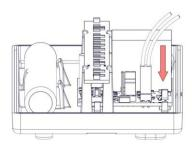
6 Connect the battery's cable with the appropriate terminal.
