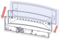
7 Refit carefully the removed plastic parts and power on the device.
