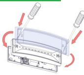
Dismantle the device carefully by using a flat bladed screwdriver.
