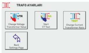
In this page you can start the current transformer test and change the current transformer and voltage transformer value.
