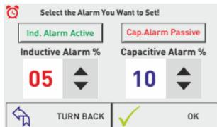
In this page inductive/active and capacitive/active Alarm mode can be made passive or active and inductive/active and capacitive/active ratio can be set. When the setting is active color of the button's writing becomes green, when it is passive it becomes red. When the ratios rise above the activated set value, the display shows "High Inductive" or "High Capacitive" warning. Also "ALR1" is on. When the Alarm mode is passive, the display doesn't show warning.
