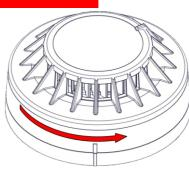
Remove the detector from its base by rotating counter-clockwise till the side marks are aligned.
