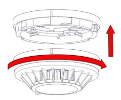
Place the detector carefully so that the side marks are aligned and rotate the detector clockwise until it locks. Provide power to the device and after 3-5 seconds it is ready for operation.
