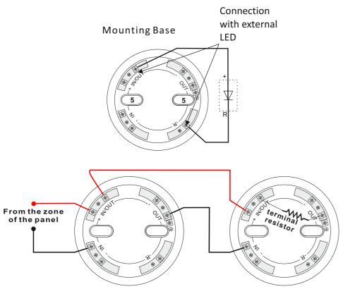
Connect the power cables (minding the correct polarity) according to the requirements of the installation.
