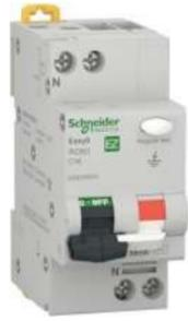
Residual current breaker with overcurrent protection (RCBO), Easy9, 1P+N, 10A ;16A ;20A ;25A ;32A, C curve, 4500A, AC type, 30mA
