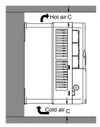
Figure 4-4 Parallel installation
