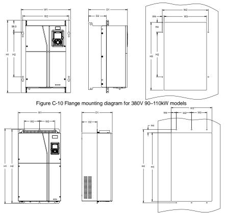
Figure C-11 Flange mounting diagram for 380V 132–200kW models
