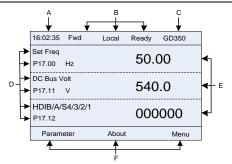
Figure 5-2 Main interface of LCD
