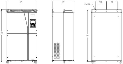
Figure C-7 Wall mounting diagram for 380V 132–200kW models
