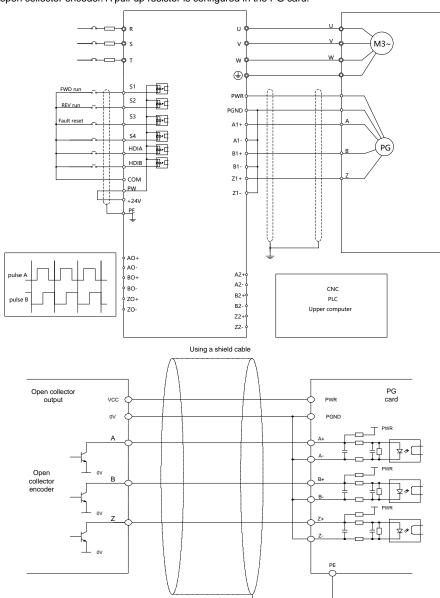
The following figure shows the external wiring of the PG card when it is used in combination with a push-pull encoder.
