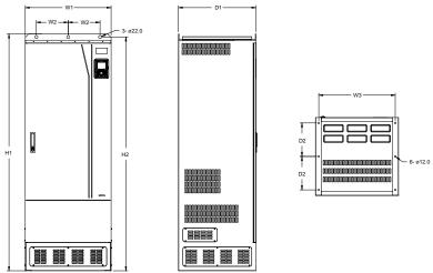
Figure C-20 Floor mounting diagram for 660V 400-630kW models
