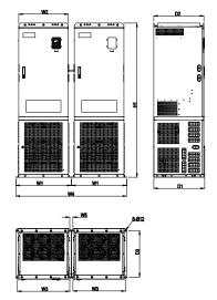
Figure C-22 Parallel mounting diagram for 380V 710-3000kW and for 660V 800-3000kW
