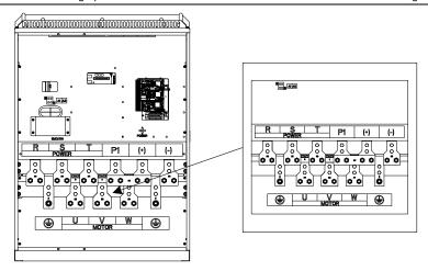
Figure 4-15 380V 220-315kW (without Al1 or Al2) and 660V 250-355kW
