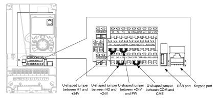
Figure 4-19 Position of U-shaped jumper
