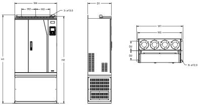
Figure C-19 Floor mounting diagram for 660V 250-355kW models
