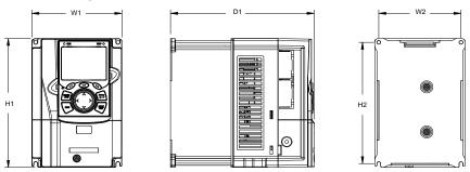
Figure C-4 Wall mounting diagram for 380V 1.5-37kW models
