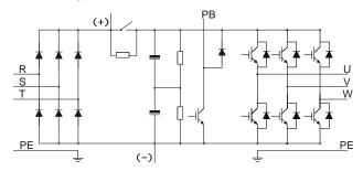
Figure 3-1 380V (15kW and lower) main circuit diagram
