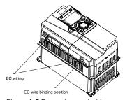
Figure A-5 Expansion card wiring
