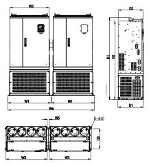
Figure C-21 Parallel mounting diagram for 380V 560-630kW and for 660V 710kW
