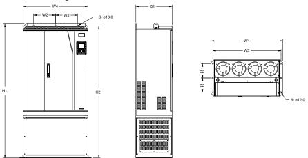
Figure C-12 Floor mounting diagram for 380V 220–315kW models
