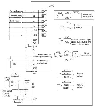
Figure 4-18 Wiring diagram of control circuit
