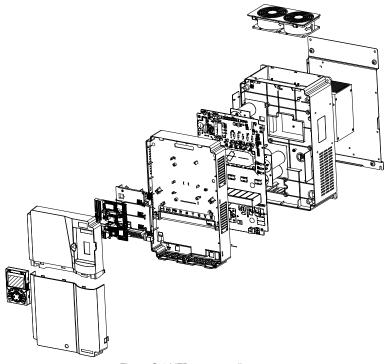
Figure C-3 VFD structure diagram
