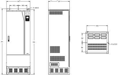
Figure C-13 Floor mounting diagram for 380V 355-500kW models
