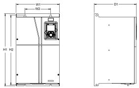
Figure C-6 Wall mounting diagram for 380V 90-110kW models
