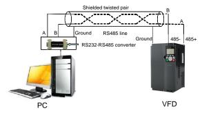
Figure 9-1 Wiring of RS485 applied to one VFD
