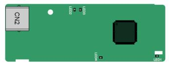
The EC-TX504 communication card adopts standard RJ45 terminals. It is used only on the upper computer that supports INVT Workshop. If you want to support the standard EtherNet/IP protocol, select the card EC-TX510.
