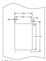
Figure C-9 Flange mounting diagram for 380V 1.5-75kW models
