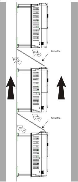
Figure 4-5 Vertical installation
