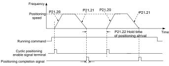
P21.25 Hold time of positioning completion signal
