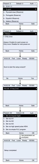
Figure 5-22 Power-up setup wizard
