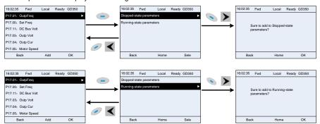
Figure 5-13 Adding parameter diagram 1
