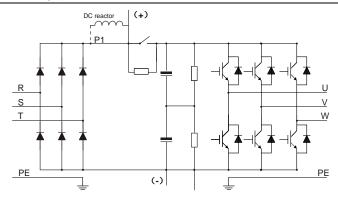
Figure 3-3 380V (132kW and higher) main circuit diagram
