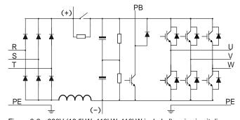
Figure 3-2 380V (18.5kW-110kW, 110kW included) main circuit diagram
