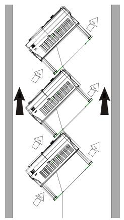
Figure 4-6 Tilted installation
