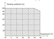
**Note:** It is not recommended to use the VFD at an environment with the temperature higher than 50°C. If you do, you shall be held accountable for the consequences caused.
