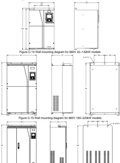
Figure C-16 Wall mounting diagram for 660V 250–355kW models
