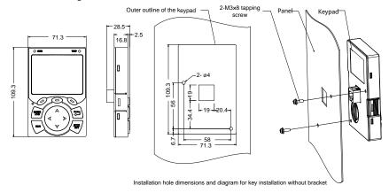
Figure C-1 Keypad structure diagram
