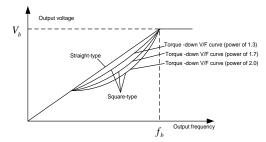
The VFD also provides multi-point V/F curve. You can alter the V/F curve outputted by VFD through setting the voltage and frequency of the three points in the middle. The whole curve consists of five points starting from (0Hz, 0V) and ending in (fundamental motor frequency, rated motor voltage). During setting, follow the rule:  $0 \le f1 \le f2 \le f3 \le Motor$  fundamental frequency, and,  $0 \le V1 \le V2 \le V3 \le Motor$  rated voltage
