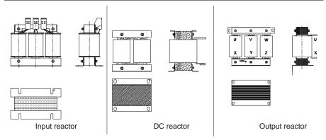
Figure D-1 Vertical reactor diagram for 380V 315kW and lower and 660V 350kW and lower
