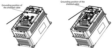
Figure A-4 Expansion card grounding diagram
