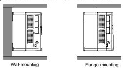
Figure 4-2 Installation mode
