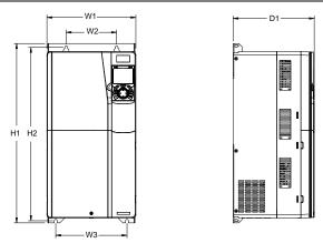
Figure C-5 Wall mounting diagram for 380V 45-75kW models
