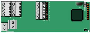
SW1 is the start/stop switch of the programmable expansion card. CN1 contains terminals PE, 485-,
