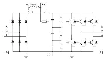
Figure 3-4 660V main circuit diagram
