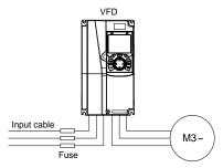
Figure 4-22 Fuse configuration
