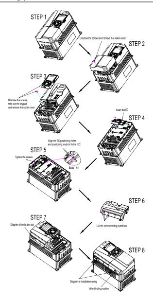
Figure A-3 Expansion card installation process diagram
