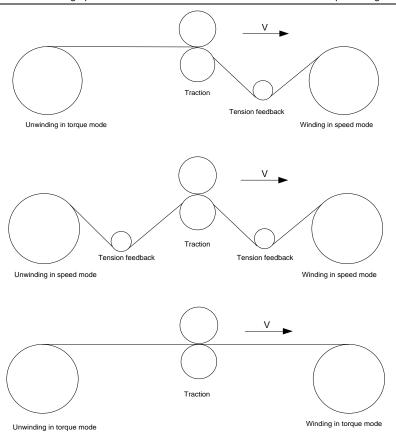
In some special situations, if the roll diameter can be counted through thickness, the following applications can be implemented:
