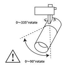
Please adjust the illumination angle of the lamp when it is not powered on.
