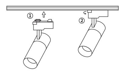
Install the track connector into the track, and rotate the track head to snap over the snap point. Make sure the conductors are fully contacted.
