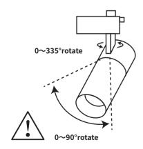
Please adjust the illumination angle of the lamp when it is not powered on.
